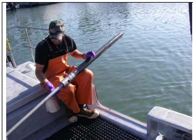
Figure 12. Piston Core Sampling
